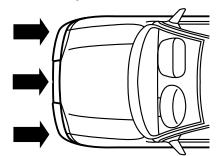
cause activation. Front airbags are designed to activate in frontal and near-frontal collisions, not rollover, side-impact, or rear-impacts unless the collision causes sufficient longitudinal deceleration.
